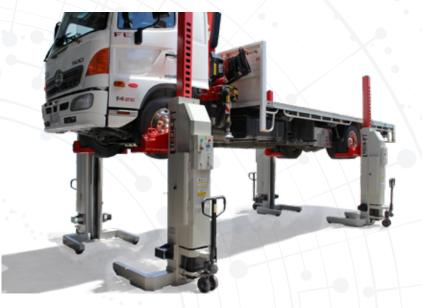
Easy access buttons Each column features operation & emergency buttons for ease of access.
